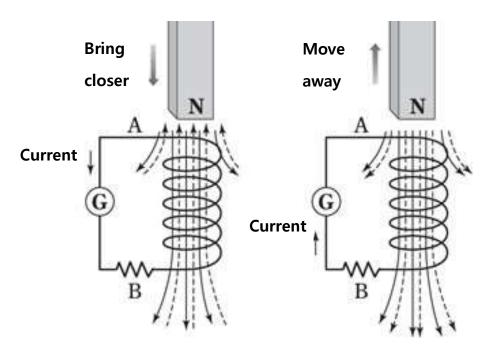
The direction of the induced EMF is such that it opposes the change in magnetic flux that caused it. If the magnetic flux through the solenoid increases, the induced EMF will create a current that generates a magnetic field opposing the increase. Conversely, if the magnetic flux decreases, the induced EMF will create a current that generates a magnetic field opposing the decrease.
